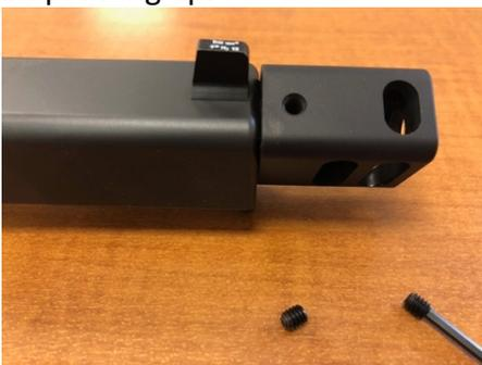
Back off the comp to align the ports pointing up. This will also give you a clearance gap between the slide and comp which is very important. Make sure they do not come into contact with each other and there is a gap between the comp and slide.
