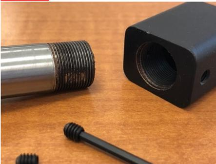
Install the barrel into the slide in the locked position, but do not install the guide rod/spring or frame (it will get in the way). Screw the comp on until it bottoms out on the end of the slide. Rarely, if ever, will the ports be pointing up.
