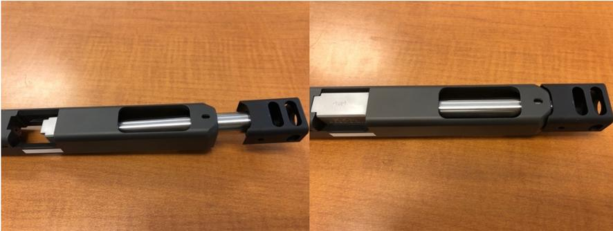
Once aligned and set, reinstall the set screws and hand torque with the little hex-wrench provide. Feel free to torque away as you will not hurt the barrel, comp, or set screws. The little wrench will bend or twist before you hurt anything else. Again, keep the set screws dry and do not use Loctite on the barrel threads.
